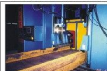
HATALY HGB1575MS H型鋼高精度重切削開銑機
